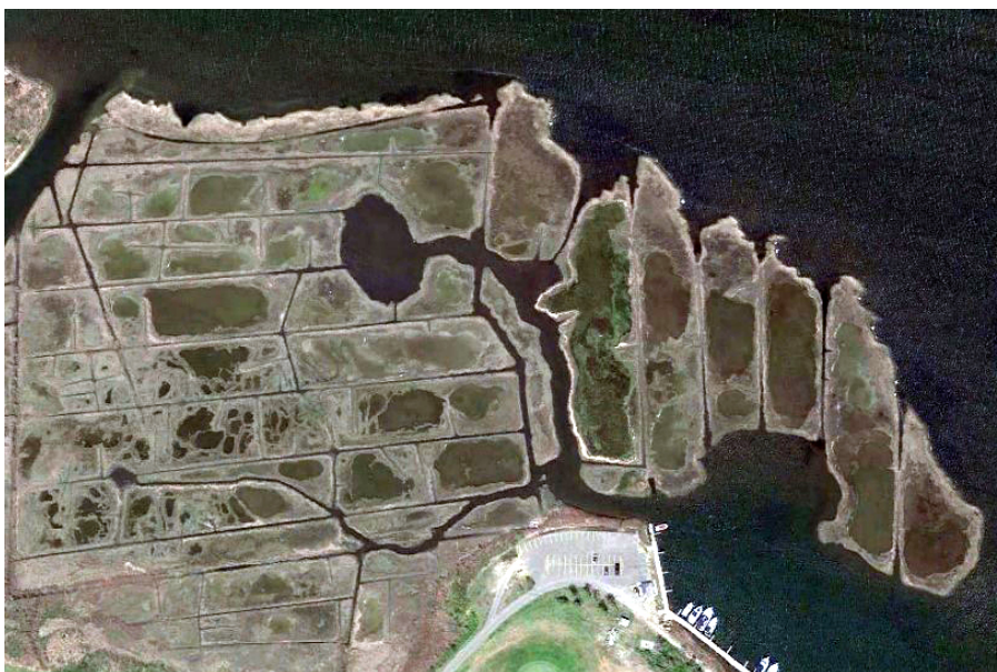
FIGURE 4. Marsh ponding between ditches, Great River, Suffolk County, NY. Hydrological restoration is planned at this site. Tidal range, 0.34 m. (Source Imagery © Google Earth.)
