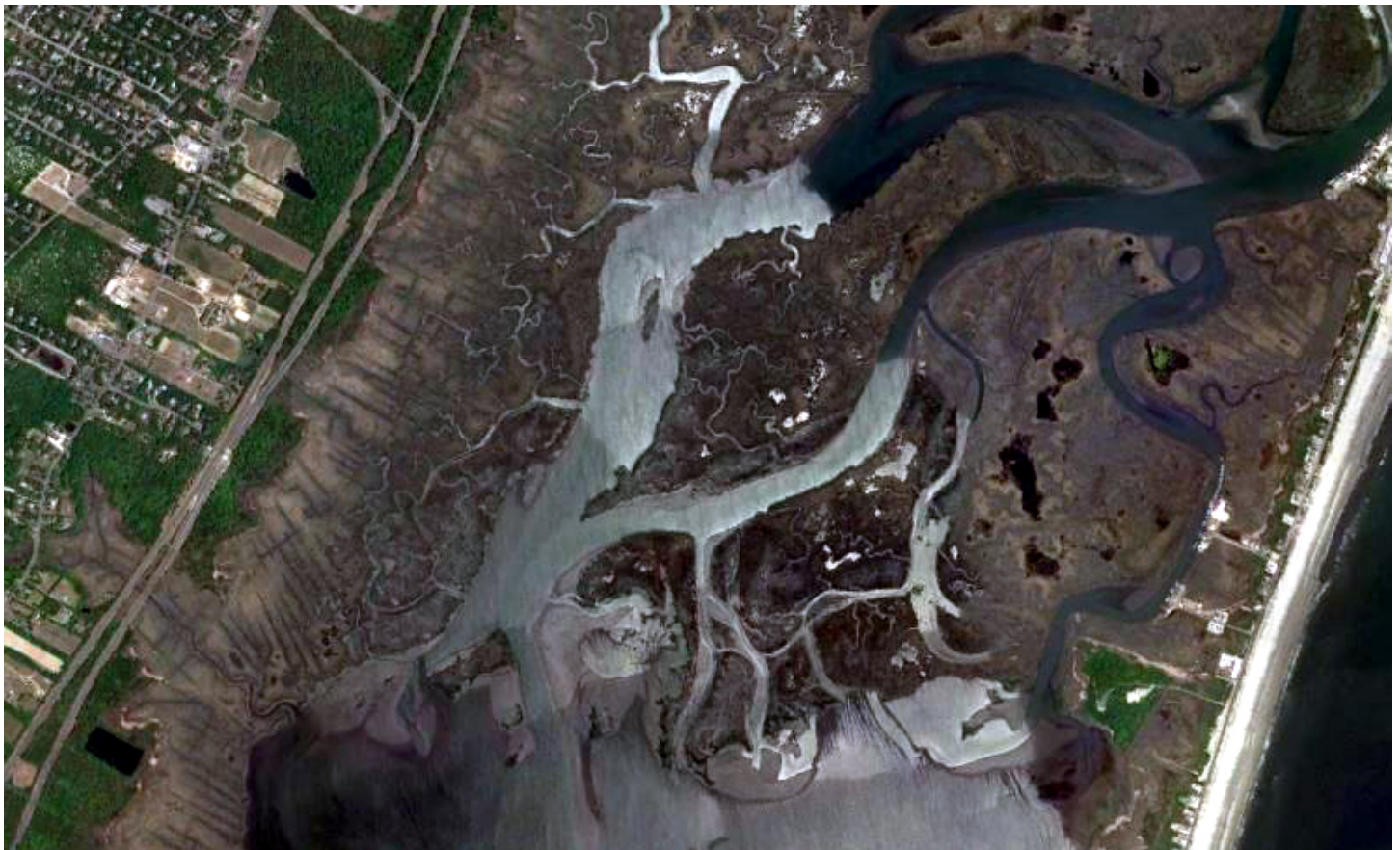
FIGURE 7. Marshes between barrier islands and the mainland in southern New Jersey. Notice the ditched sections along the mainland and the barrier island, while large sections of relatively unaltered marshes are surrounded by open water. (Source Imagery © Google Earth.)
