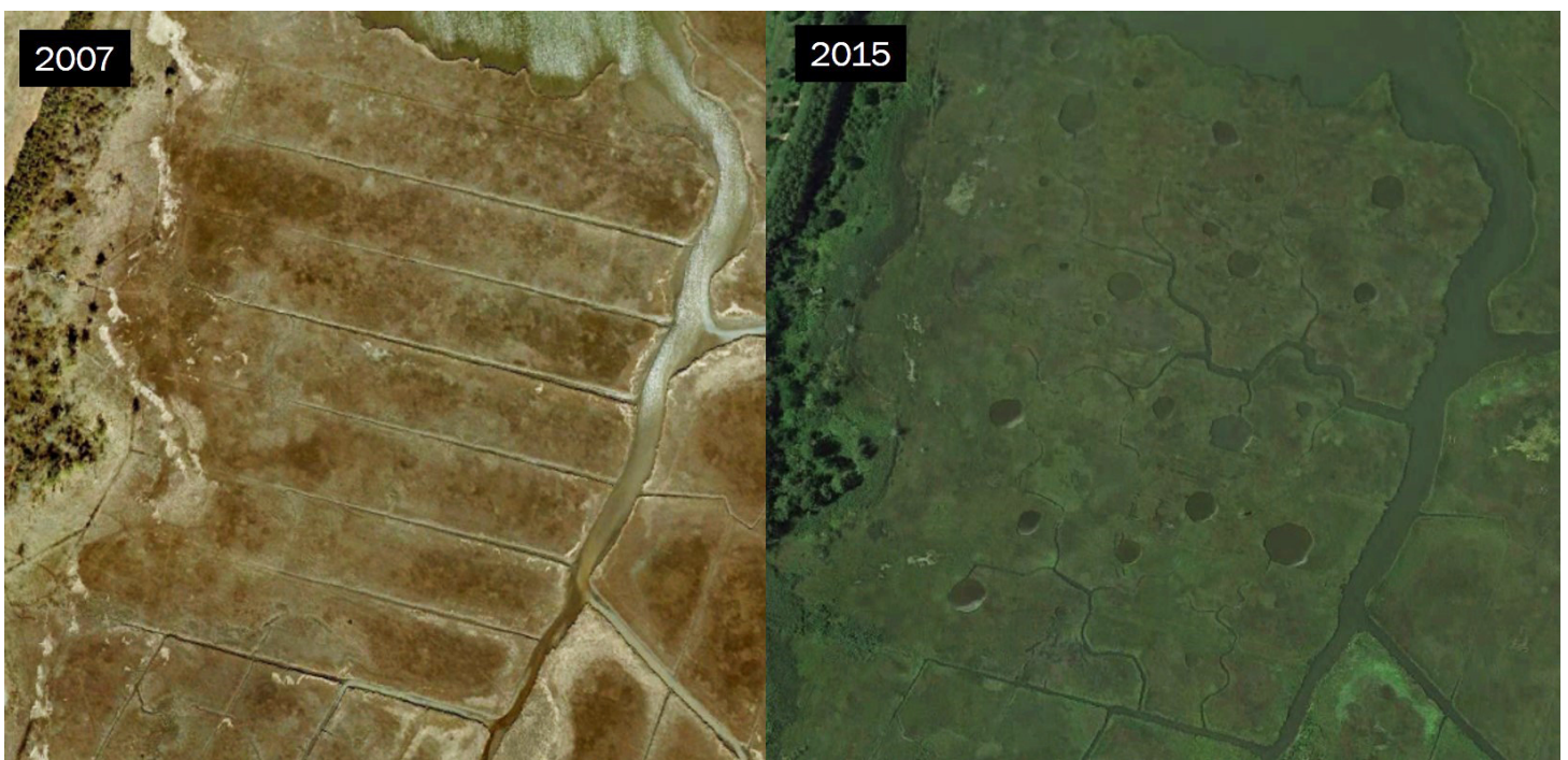
FIGURE 6. Sloughs Gut Project (Delaware) restored natural tidal marsh hydrology without sediment addition including breached and unbreached pools to a grid-ditched marsh. Tidal range 0.75m. (Source Imagery © Google Earth.)
